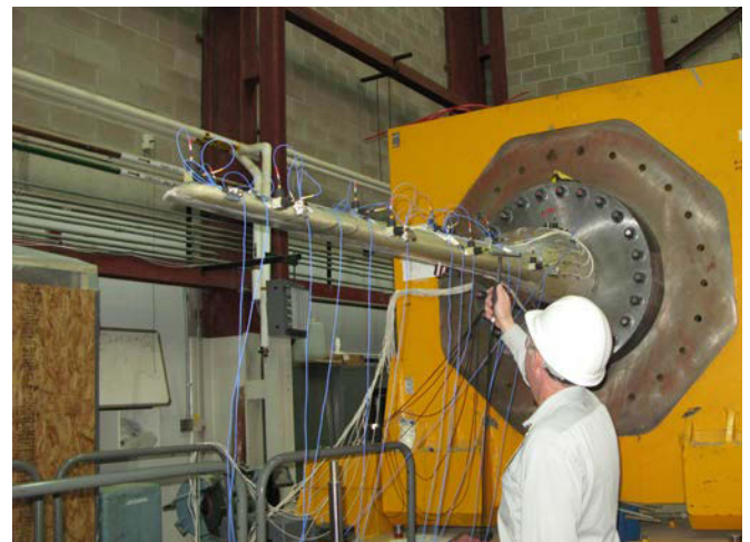
Low-pressure surface view of structural validation of the Verdant 56-kW Composite KHPS Blade at NREL. Photo by Mike Desmond, NREL 21715
