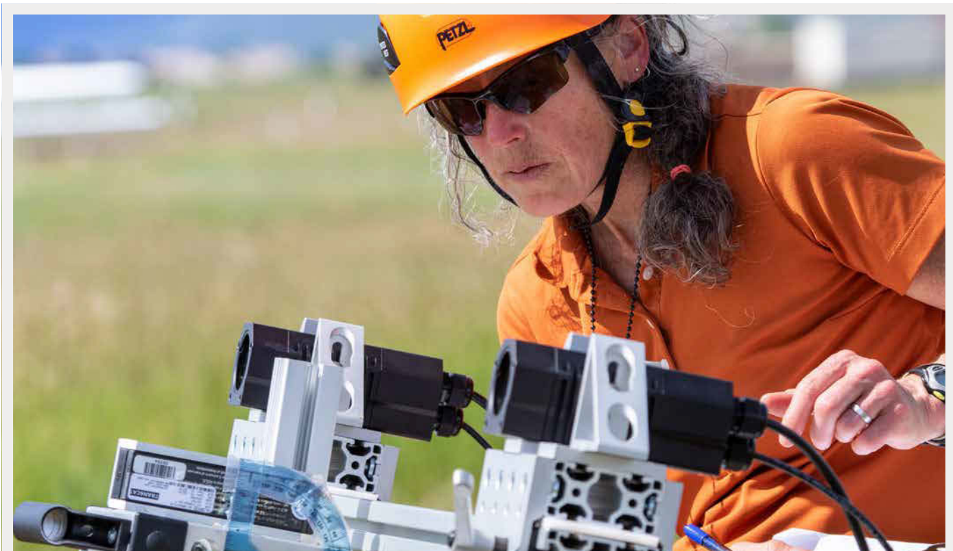
Time for a checkup. Stereoscopic vision from ThermalTracker provides more accurate tracking of wildlife. Photo by Werner Slocum, NREL
