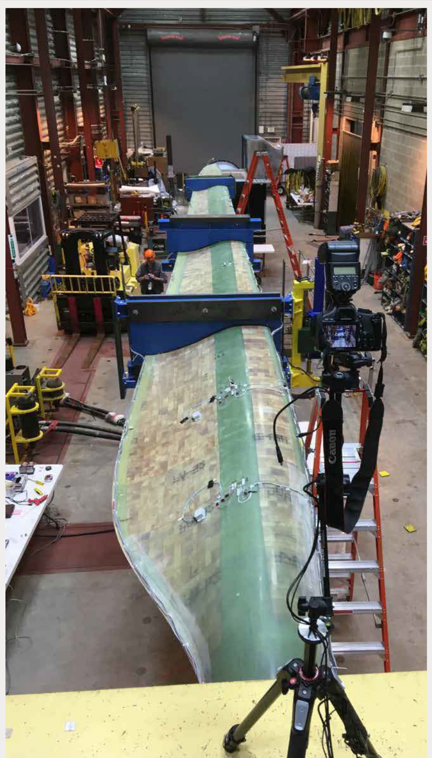
Preventive health for wind turbine blades. Sentient Science's wind blade fatigue assessment in NREL's Structural Testing Laboratory includes a 13-m blade and an optical measurement system, shown on top of the test stand. Photo by Ryan Beach, NREL
