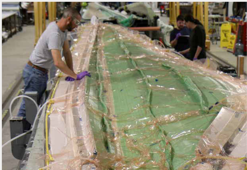
The team works to develop a blade using recyclable thermoplastic material. Photo by Dave Snowberg, NREL
