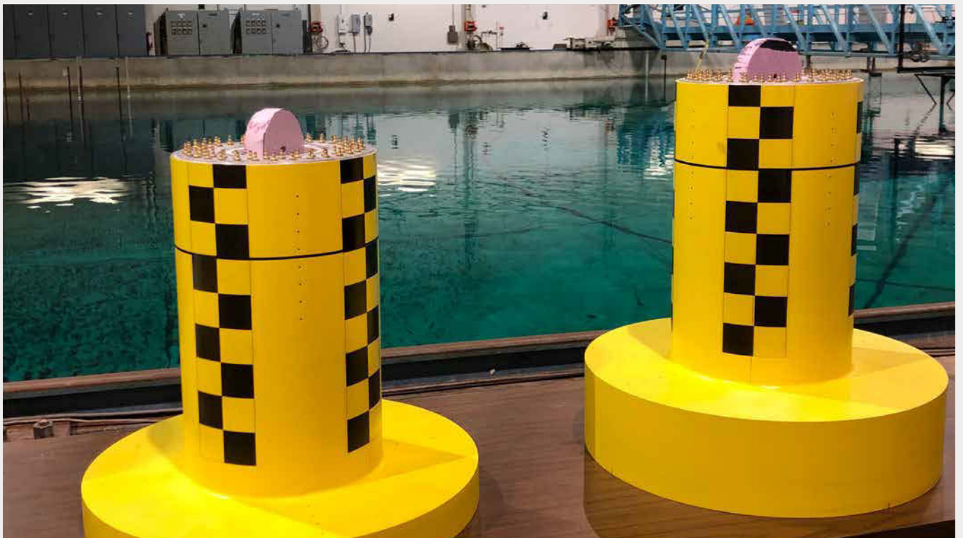
As part of the OC6 tank test, cylinders with heave plates attached to the bottom were individually validated to gather data to better understand the physics that interact on different components of an offshore wind system. Photo by Amy Robertson, NREL
