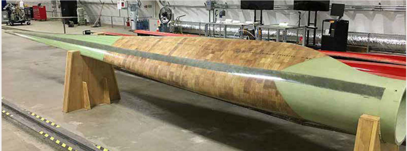
Green blade for green enterprise. NREL researchers are currently validating a 13-m thermoplastic composite wind blade at the Structural Technology Laboratory. A report comparing the structures of a thermoplastic composite wind turbine blade and a thermoset composite wind turbine blade will be published soon. Photo by Dave Snowberg, NREL
