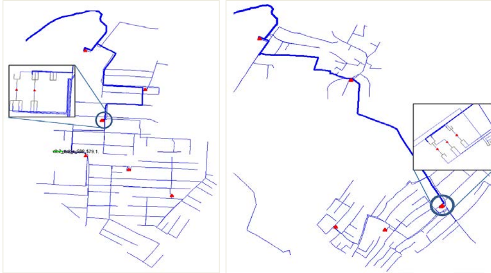
Figure 20. Feeder models showing the primary and secondary networks separated by the distribution transformers (red triangles)
