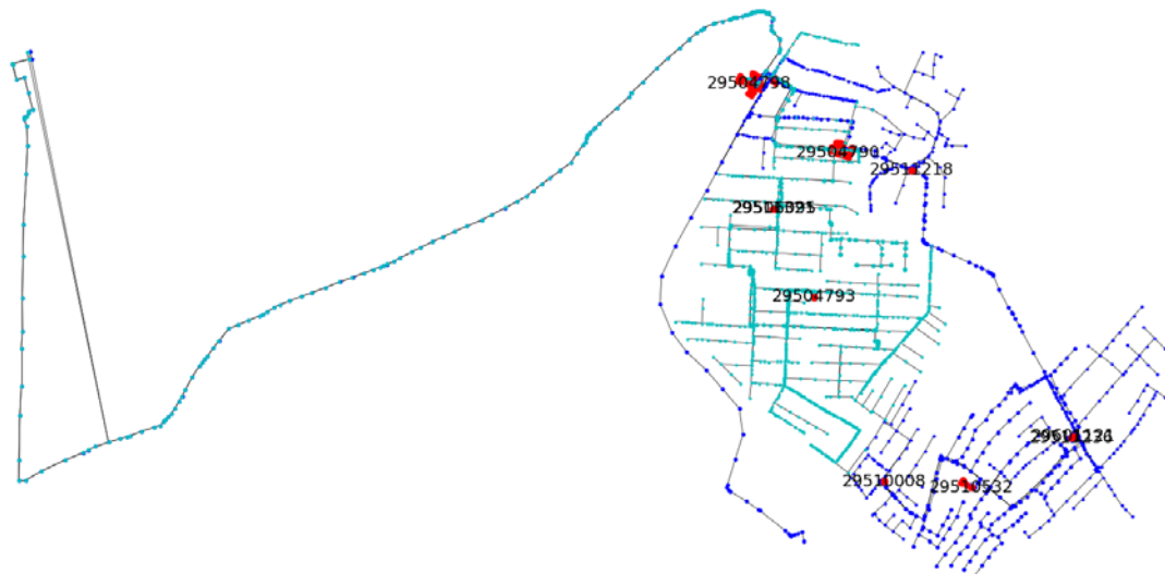
Figure 85. Line loading relief as a result of BESS integration under the high EV penetration scenario
