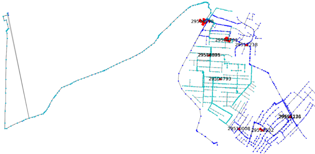
Figure 64. Line loading relief as a result of BESS integration under the high EV penetration scenario
