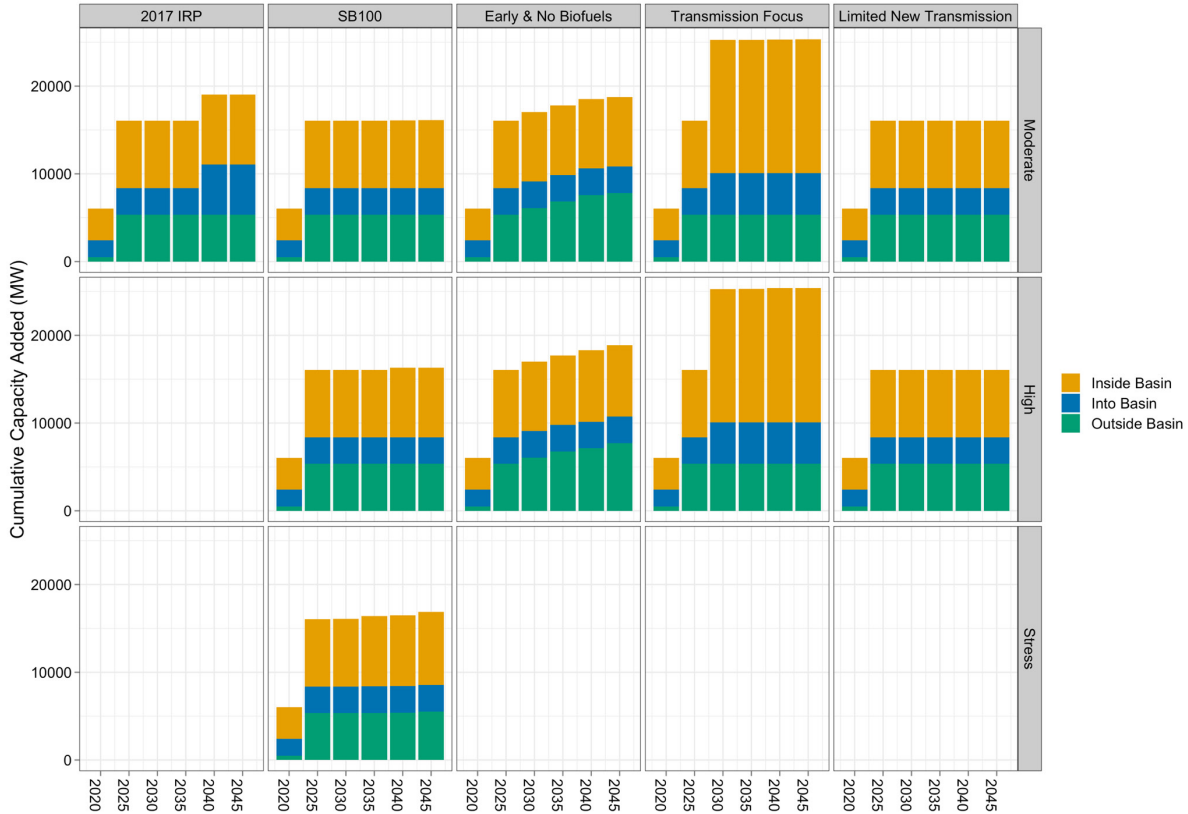
Figure 23. The combined capacity of inside-basin, into-basin, and outside-basin transmission upgrades added through 2045 for all scenarios and load projections, including existing plans for transmission, firm as of June 2020 and communicated by LADWP
