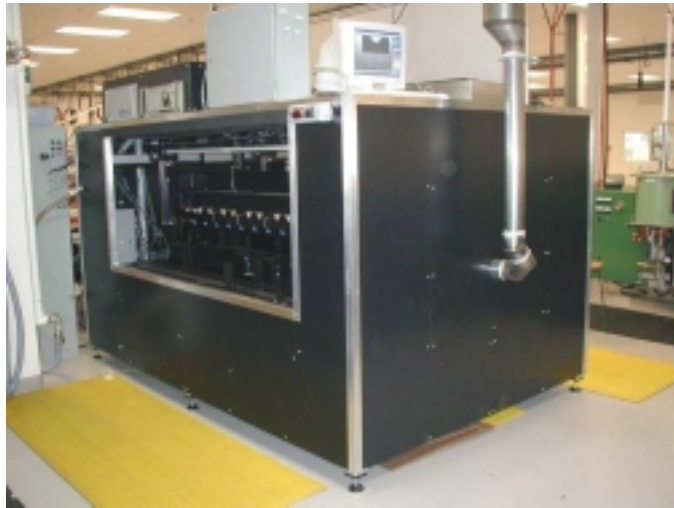
Figure 9 Automated Laser Cutting Machine.
