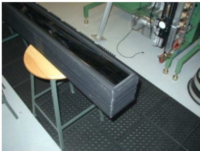
Figure 10 Stack of String Ribbon Strip Holders.
