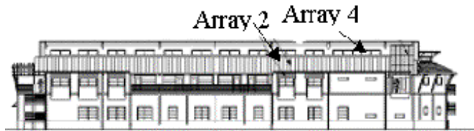
Figure 3. West elevation view of SAO with PV integrated into standing seam metal roof and curtain wall.
