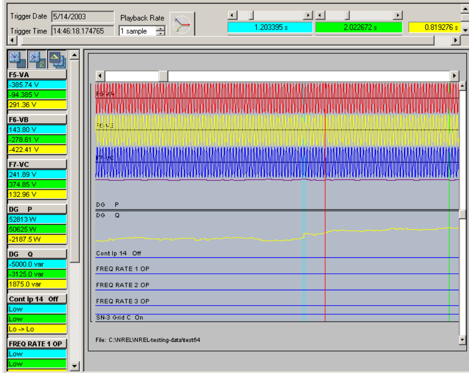
Figure 34. 10-kW resistive load step-up with base load of 50 kW, 90 kVAR L and C
