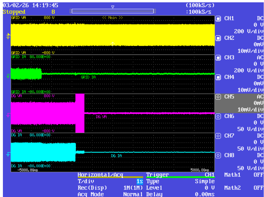
Figure 23. Over frequency trip waveforms
