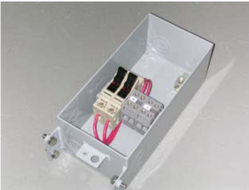
Figure 22. PVSCP-2 provides fused landing place for 2 PV source circuits, that are bussed and pre-wired to output lugs. Source circuit wiring enters through strain relief connectors (not shown) in knockouts on side of box.
