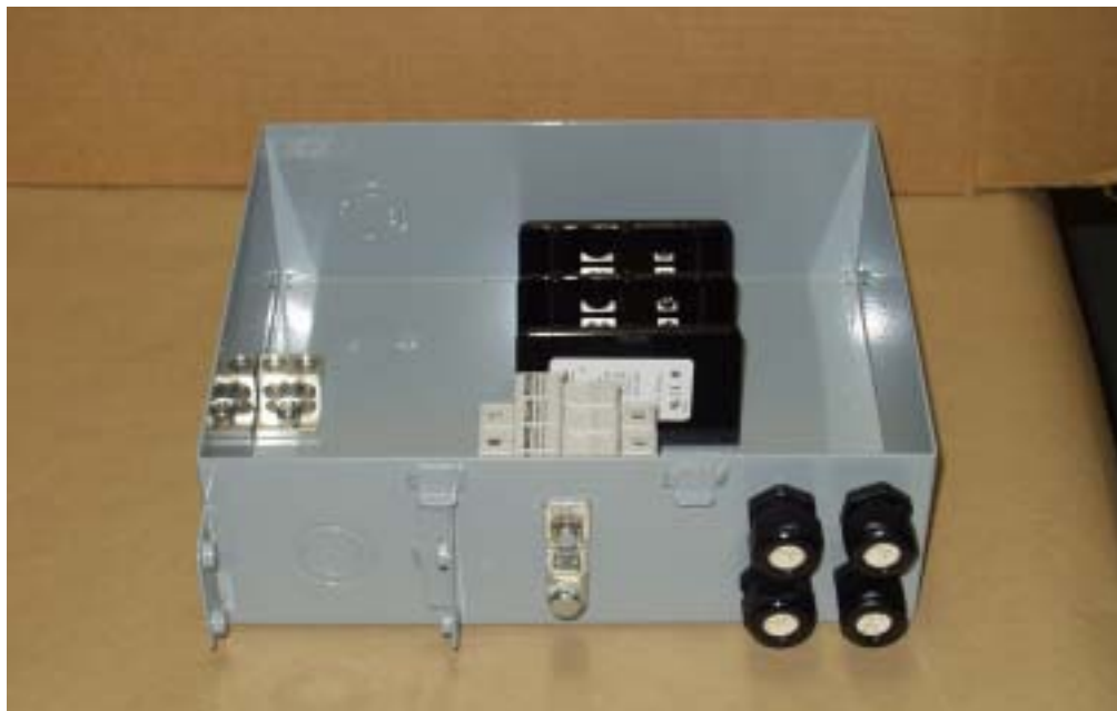
Figure 20. PVSCP-4, showing four 2-hole strain relief connectors through which the positive and negative conductors from 4 PV source circuits enter the box. Note external and internal ground lugs for termination of equipment ground wires.
