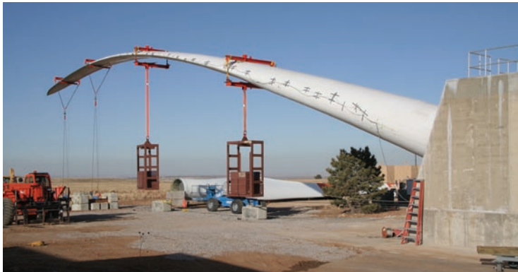
NREL conducts a static bending test on a 47-m blade using a 50-m test stand at the National Wind Technology Center, near Boulder, Colorado.
