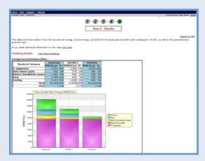
The final step in the DC Pro Profiling Tool process is the results screen, shown above. The tool generates a customized printable report that details:
