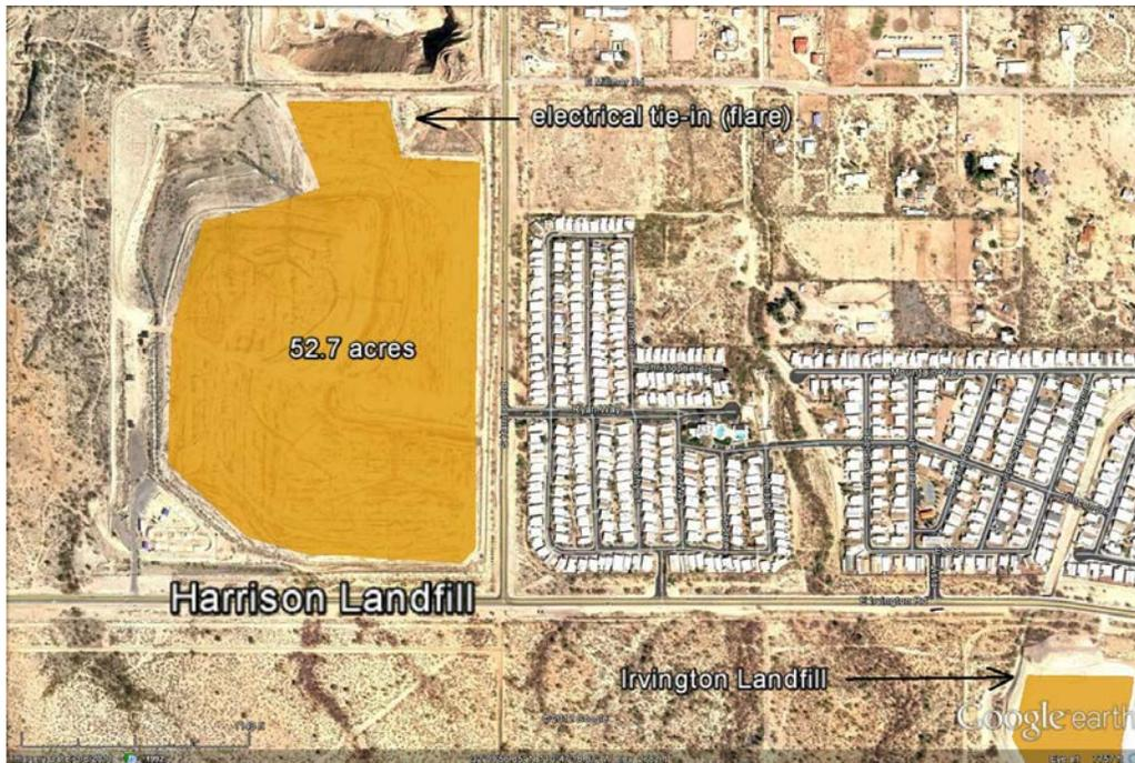
**Figure 5. Aerial view of the feasible area for PV at the Harrison Landfill**
