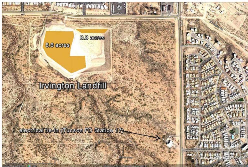
**Figure 6. Aerial view of the feasible area for PV at the Irvington Landfill**
