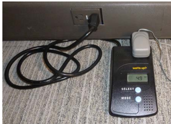
Figure 17. Temporary metering of a plug load device (Courtesy Scott Schuetter, Energy Center of Wisconsin)
