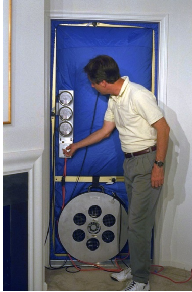
Figure 6. Fan pressure test using a blower door
