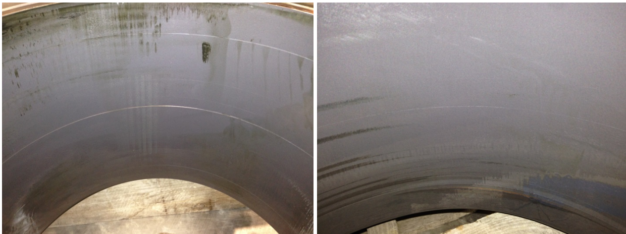
Figure 19. Journal bearing wear patterns. Photos by Jonathan Keller, NREL 36729 (left) and 36732 (right)
