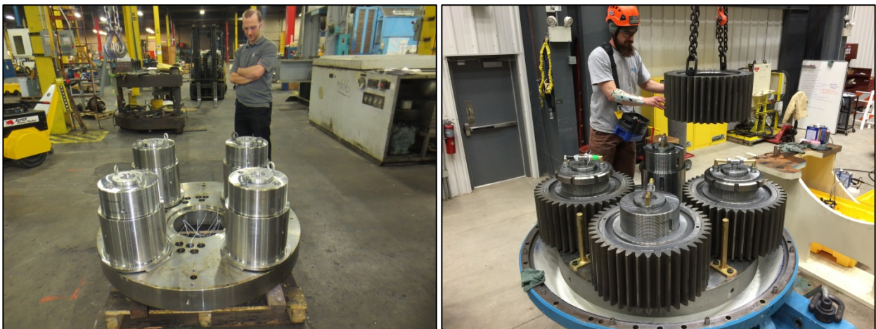
Figure 3. Planetary carrier and spindles (left) and (right) planets. Photos by Jesse Graeter, Romax Technology, NREL 33353 (left), and Jonathan Keller, NREL 33341 (right)
