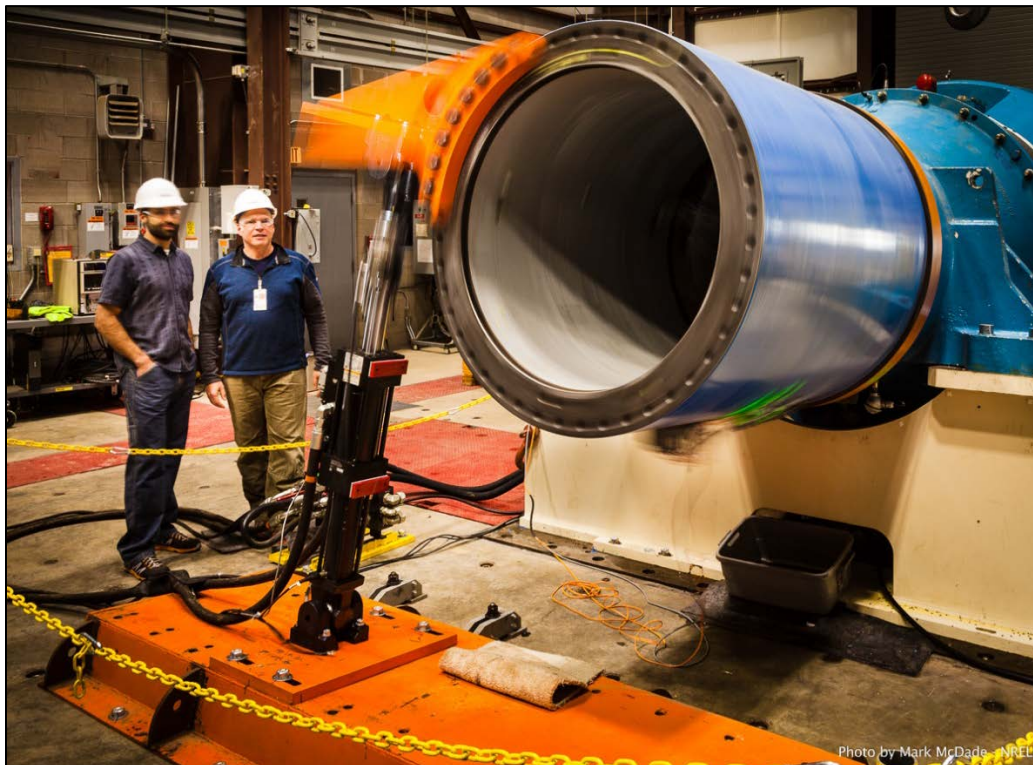
Figure 17. Unlocked and oil-restricted dither testing. Photo by Mark McDade, NREL 36517
