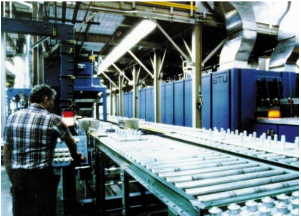
Texas Instrument's Spherical Solar™ PV technology production line.
