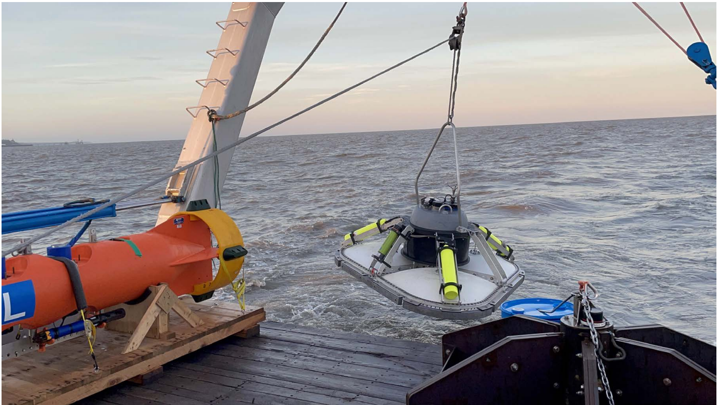
NREL researchers and crew deployed three moorings in Cook Inlet, Alaska, to collect data for a potential tidal energy site. A NEPA review was completed beforehand to evaluate potential environmental impacts of the project.. Photo by Levi Kilcher, NREL 66087
