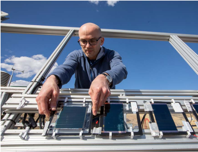
A senior scientist installs a small perovskite accelerator for solar panels at the Outdoor Test Facility at the STM Campus. Photo by Werner Slocum, NREL 67121
