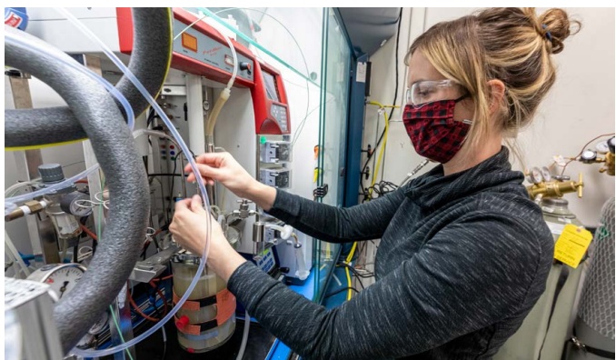
A materials and process researcher uses a fermenter to convert liquid carbon monoxide to ethanol after first converting it from carbon dioxide at the Integrated Biorefinery Research Facility. Photo by Werner Slocum, NREL 66466
