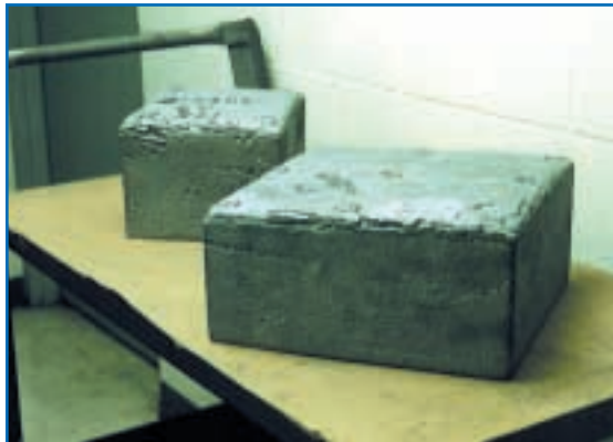
Using a process developed under PVMaT to make a larger brick of silicon doubled Solarex's PV production capacity.
