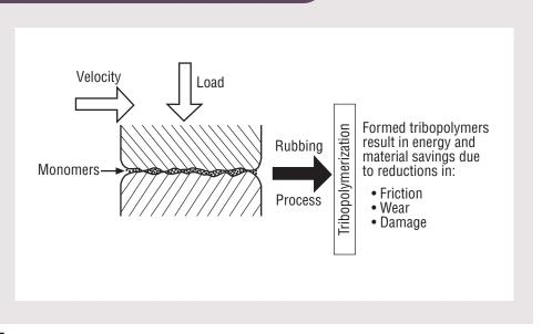
The tribopolymerization concept has led to the development of new classes of antiwear additives, which reduce friction and wear in ceramic, metal, and advanced alloy applications.
