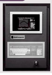
With reduced effective cost, the WeldComputer™ Resistance Welder Adaptive Control can now save energy and avoid rejects for welding operations for general commercial products such as automobiles and appliances, as well as meet the precise welding standards of the aerospace industry.
