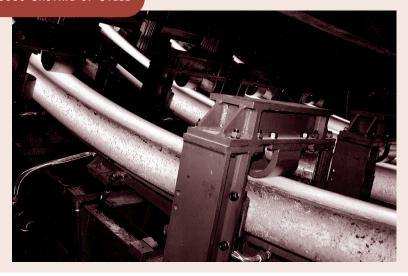
A new method for creating steel pipe and tubing combines casting and rolling of pipe into one process, reducing the amount of energy and labor required for production.
