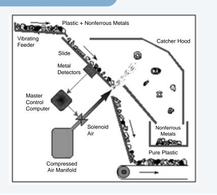
The ELPAC™ aluminum separator uses electronic eddy-current sensing and air jet pulses to separate aluminum from streams of mixed material, greatly improving the economics of plastic, glass, and aluminum recycling operations.
