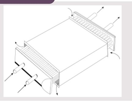
Doty Scientific's Microtube Strip (MTS) heat exchanger is smaller and more efficient than conventional heat exchangers used in power plants.
