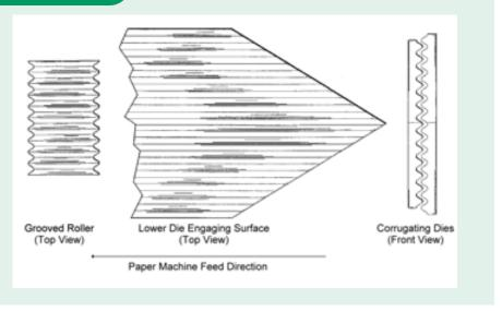
Unlike the conventional approach to producing corrugated cardboard for boxes, the new linear corrugating process uses equipment that aligns the flutes parallel to the wood fibers, imparting an estimated 25% greater crush strength to the finished product.
