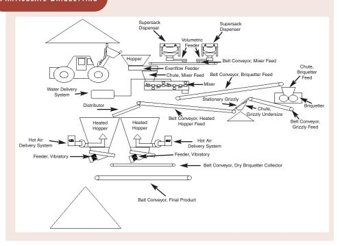
This schematic of Covol's unique system follows the steps of processing, from the loading of fine particulate by-products and other wastes with limestone or other fluxing materials, to the final step of producing stable furnace briquettes.
