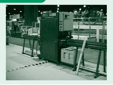
Perceptron's ultrasonic lumber inspection system scans green wood to determine if moisture levels are normal or if defects, such as "wetwood," are present.
