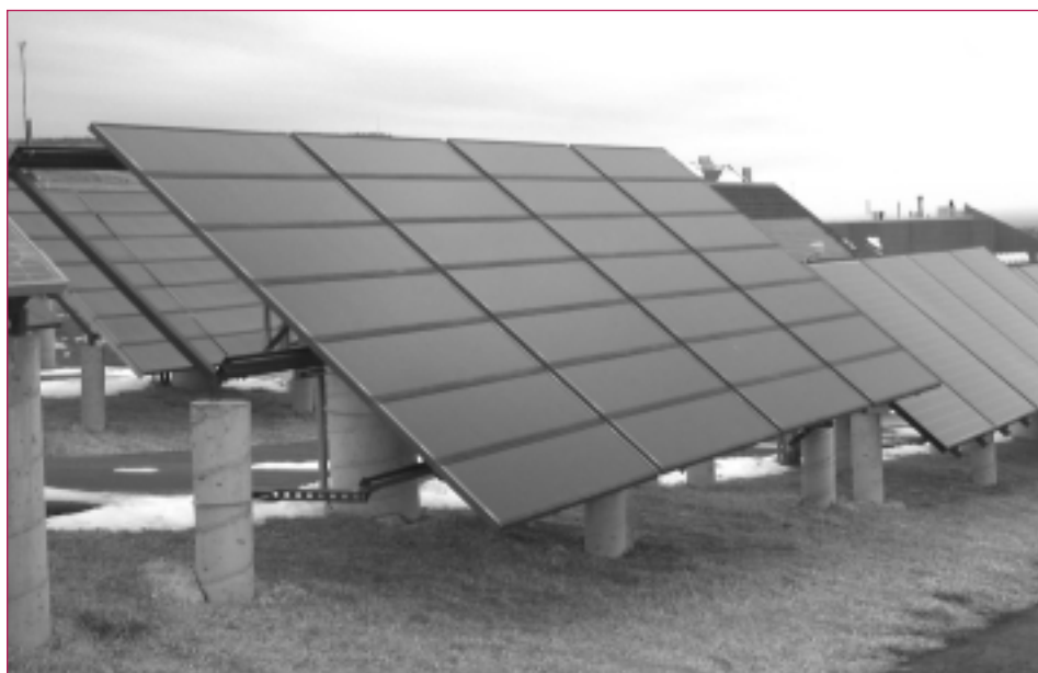
The laboratory research promise of CIS thin-film cells is proving true. This 1-kW array, comprising 28 CIS modules from Siemens Solar Industries, is the highest efficiency thin-film array to date (averaging 11.5% efficiency at Standard Test Conditions). The modules, winners of an R&D 100 Award in 1999, are being monitored at NREL for long-term performance and reliability.
