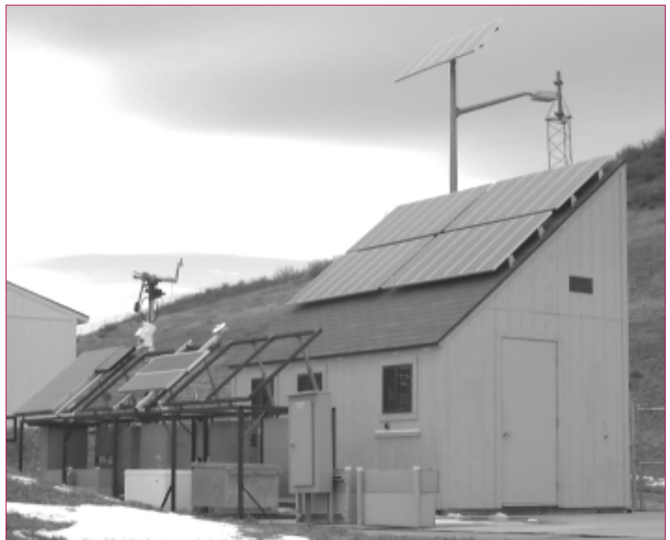
This testbed at NREL's Outdoor Test Facility can be configured in many combinations to power up to six different stand-alone systems on the front rack and one grid-connected system on the roof. The testbed was being used in 1999 to validate performance test procedures for stand-alone PV systems that could become part of the IEEE standard.
