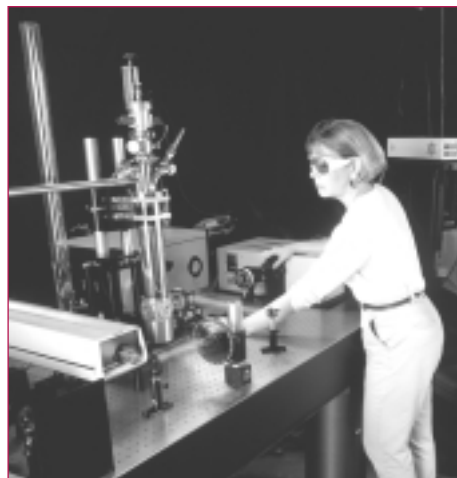
NREL uses energy-resolved photoluminescence spectroscopy to measure material quality, determine bandgaps of solid-state materials and devices, identify defects and impurities, and analyze recombination mechanisms.
