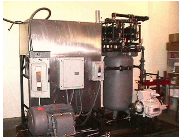
Figure 4. Compressor Test Facility with Commercial Compressor (lower right)
