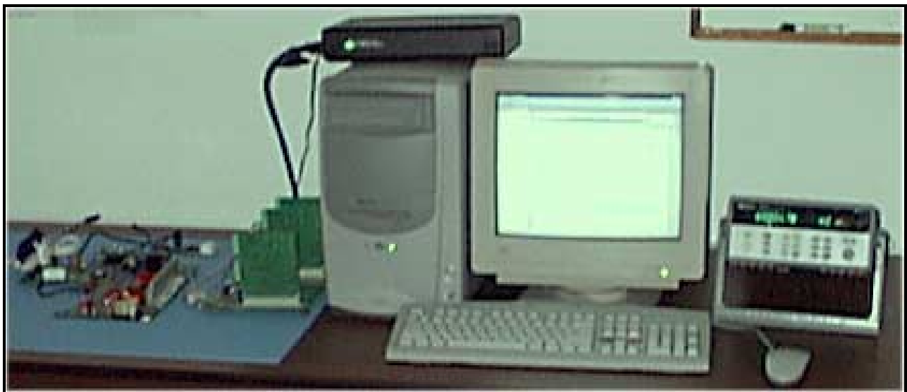
Figure 7. Burn-In Test Station (BITS) computer controls
