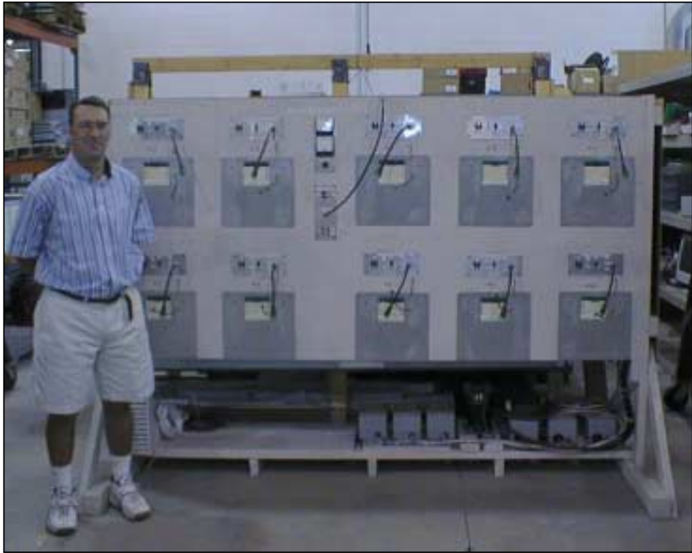
Figure 8. Burn-In Test Station (BITS).
