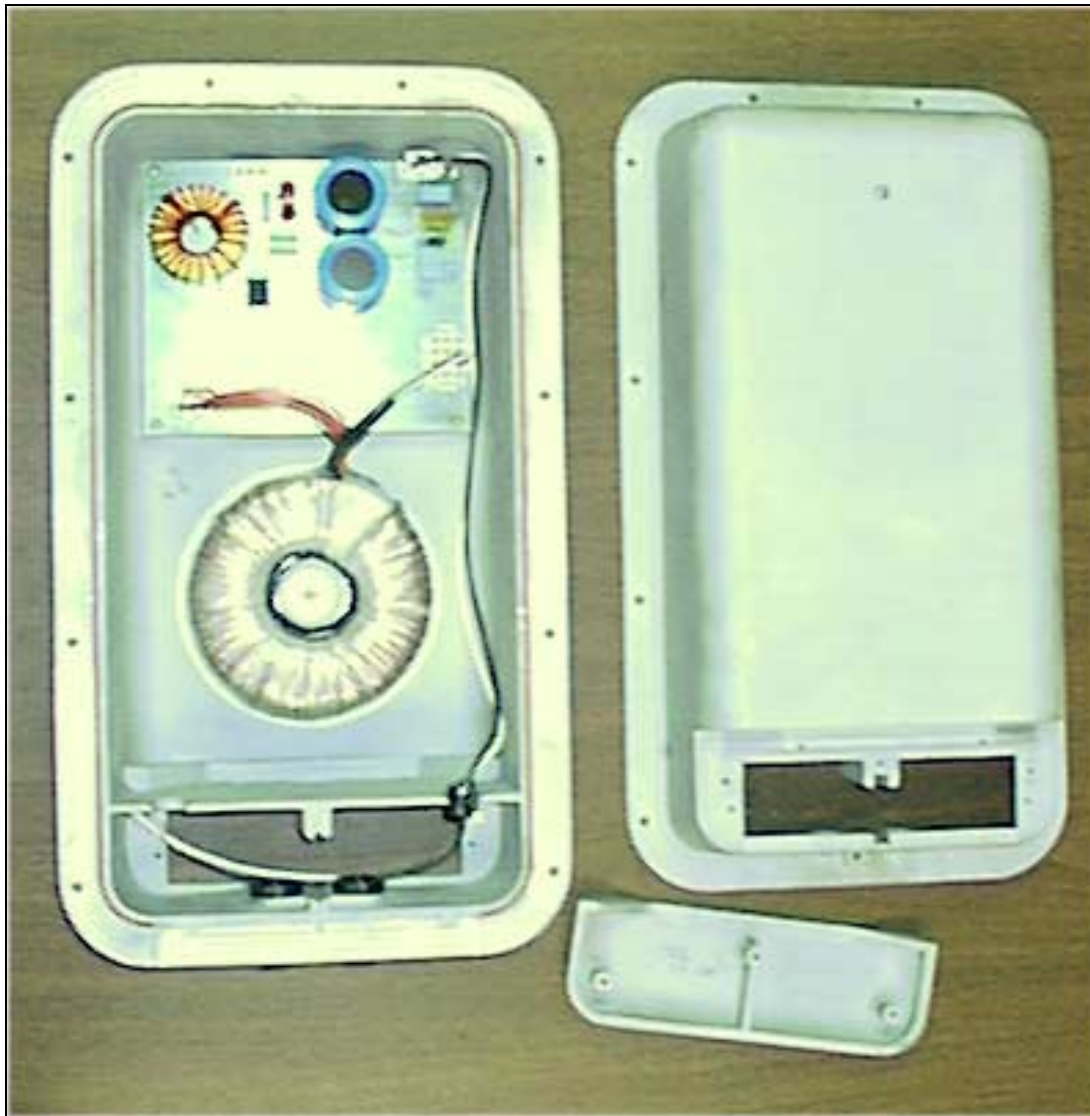
Figure 9. Picture of a prototype SunSine Inverter Assembly. Note that there is plenty of room for size reduction. The wiring compartment on the bottom will also be removed from the final design.
