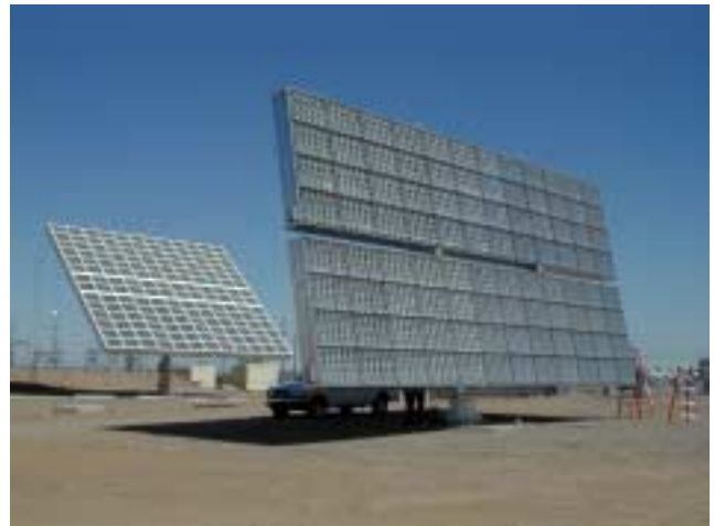
Figure 1: Two MegaModule IHCPV System
