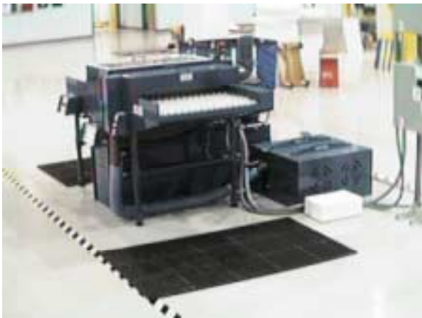
Figure 1. High throughput in-line rinser-dryer which accepts a wide range of wafers sizes.
