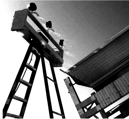
Figure 3: Photograph of a water spray station
