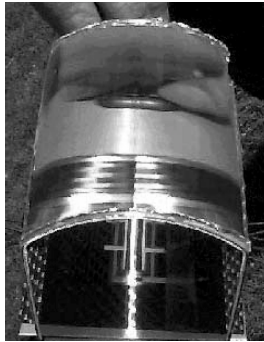
Fig. 3 - Mini-Concentrator Module Under Test Outdoors
