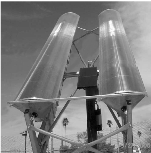
Figure 2: Photograph of a two-axis tracker with two concentrator modules installed
