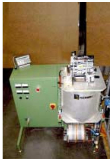
Figure 2. Furnace with ribbon growing from the machine.
