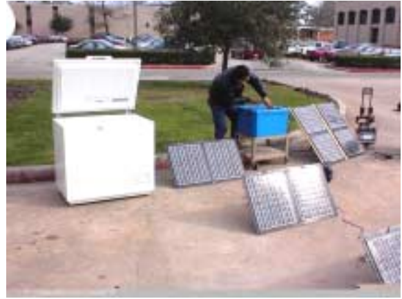
Fig. 4. The Battery Free Solar Refrigerator on Test Outside the Photovoltaic Research and Demonstration Laboratory
