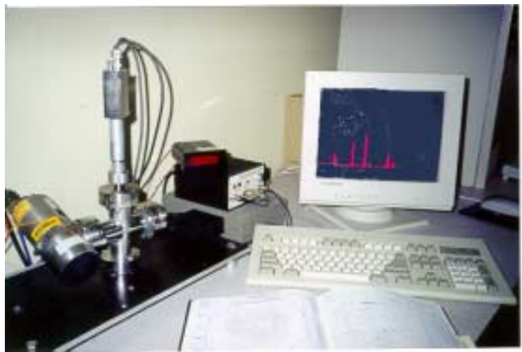
Figure 1: XRF sensor designed and assembled at MRG.
