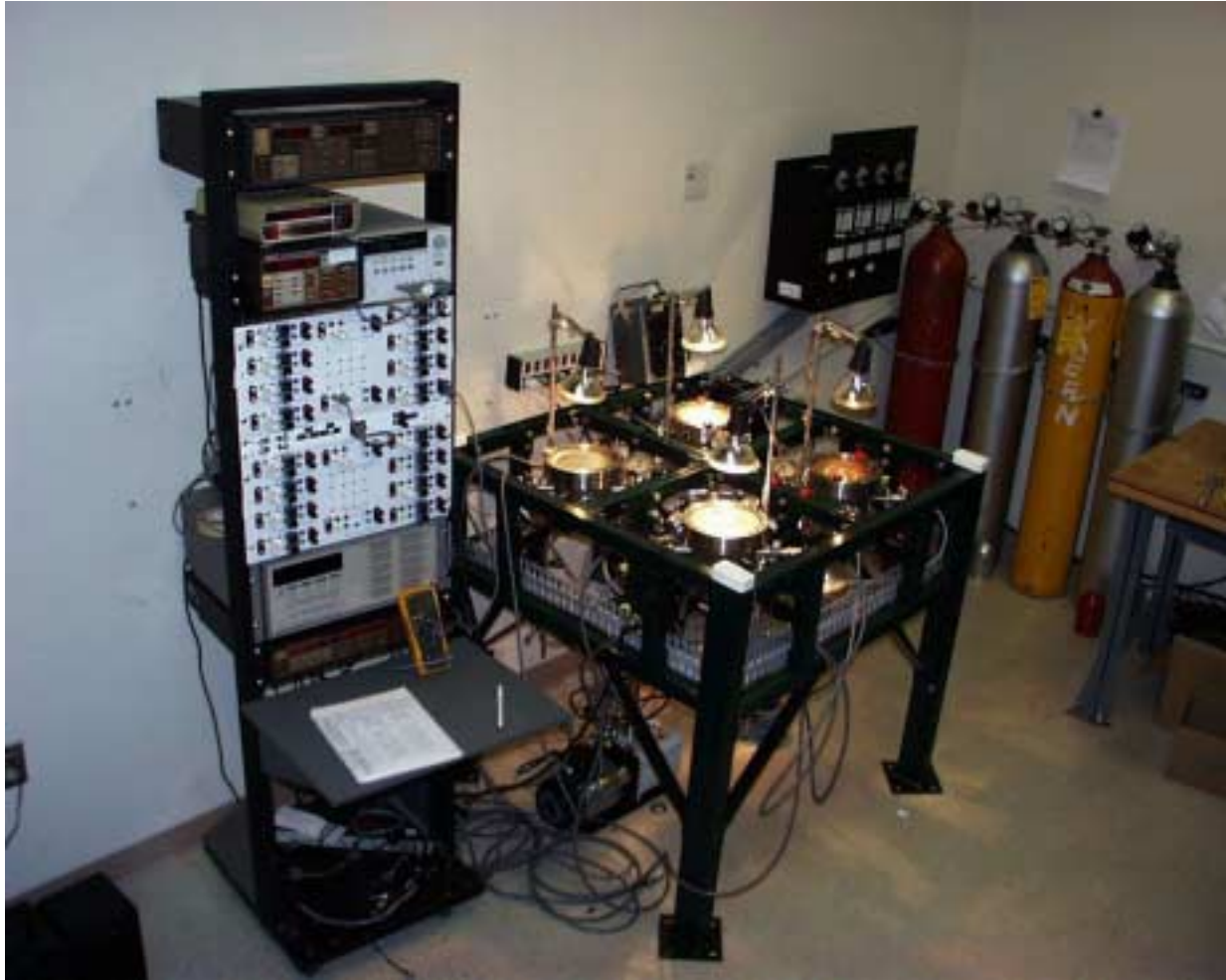
Figure 4.42 The new IEC stress testing system showing the 4 chambers with glass windows and lamps, vacuum pump, gas handling system, and bias control panel.
