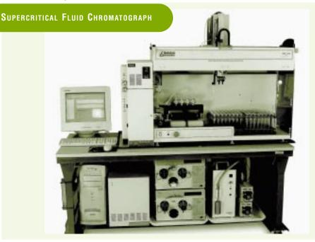
SFC technology uses CO<sub>2</sub> to achieve greater processing speed and separation of pharmaceutical compounds compared to traditional LC separation. This new type of purification improves product quality and energy efficiency, while reducing waste, processing time, and costs.
