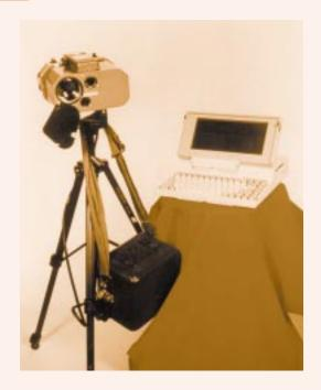
The Pulsed Laser Imager provides accurate data about volatile organic compound emissions from locations up to 1.5 miles (2.5 kilometers) away.
