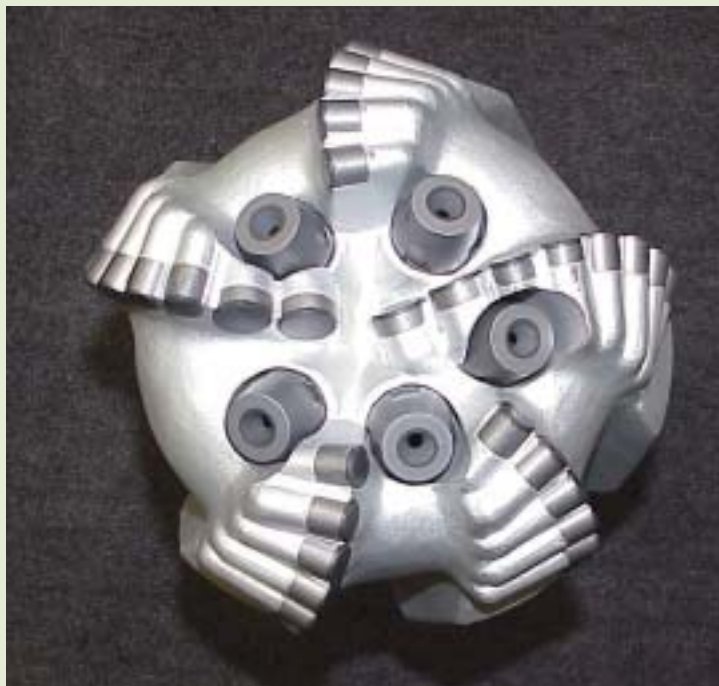
This polycrystalline diamond compact drill bit has mud-jet nozzles built into it. The photo above shows a computer model of the jets inside the bit. This photo shows a face view of the entire drill bit.
