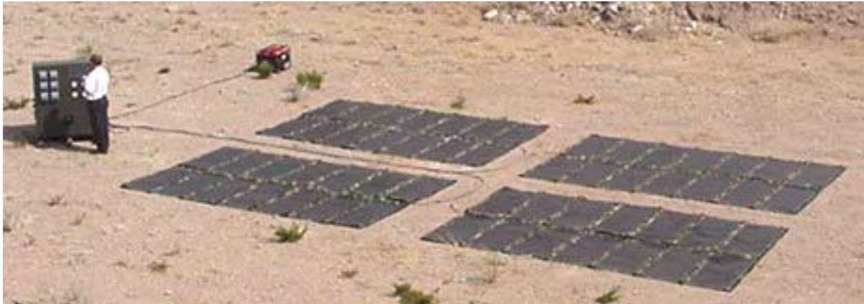
Figure 3. 3 Photograph of TACS Power Storage and Backup Generator System.
