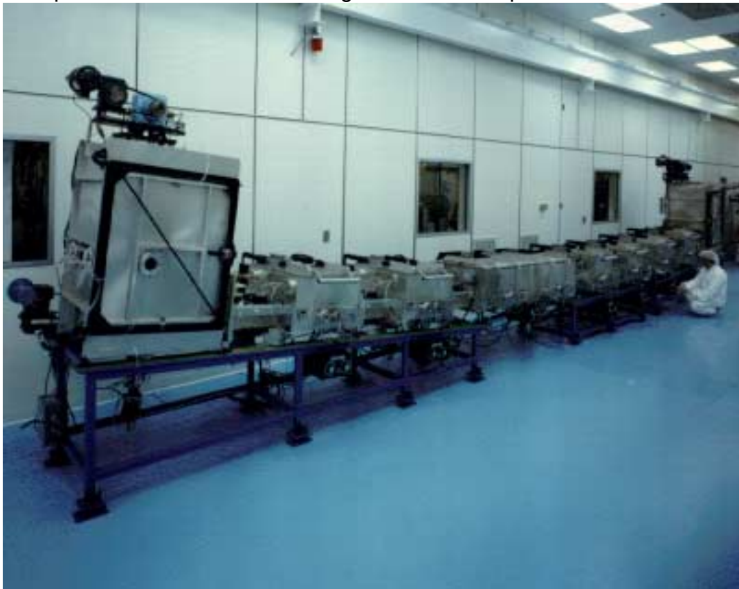
Fig. 30. Double-junction roll-to-roll plasma-CVD processor, previously used as United Solar's production machine. This machine will be used as an experimental machine for much of the work proposed in Tasks 1 and 3.
