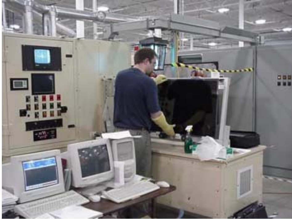
Figure 10. Photograph of First Solar rapid laser-scribing system, showing the loading station, the process control station the scribing station (enclosed in cabinet), and the power-supply station (to the rear)
