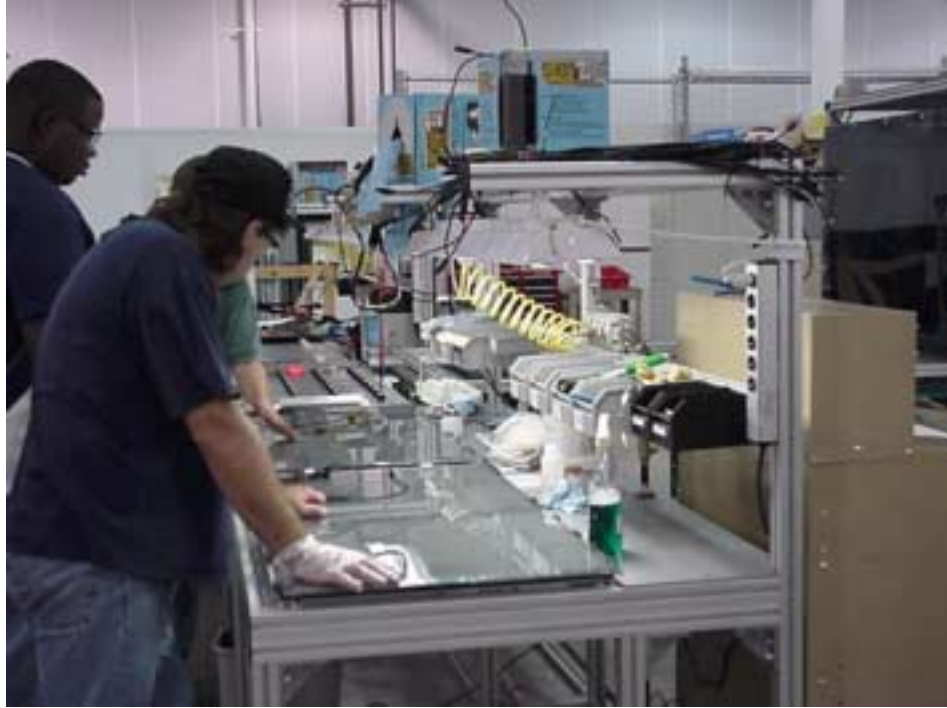
Figure 8. Cord-plate contact termination application line
