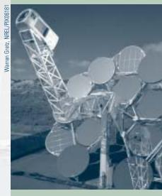
The modularity of dish systems, such as this 25-kW model manufactured by Science Applications International Corporation, makes them ideally suited to a variety of distributed power applications at home and abroad, including village electrification projects in the developing world.
