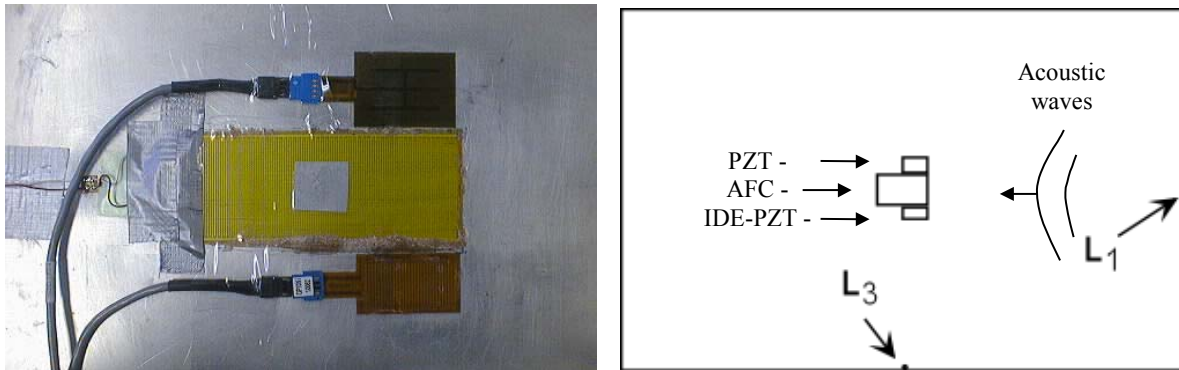
Figure 3-25. Sensor patches: (top) monolithic PZT; (center) AFC; and (bottom) PZT-IDE
