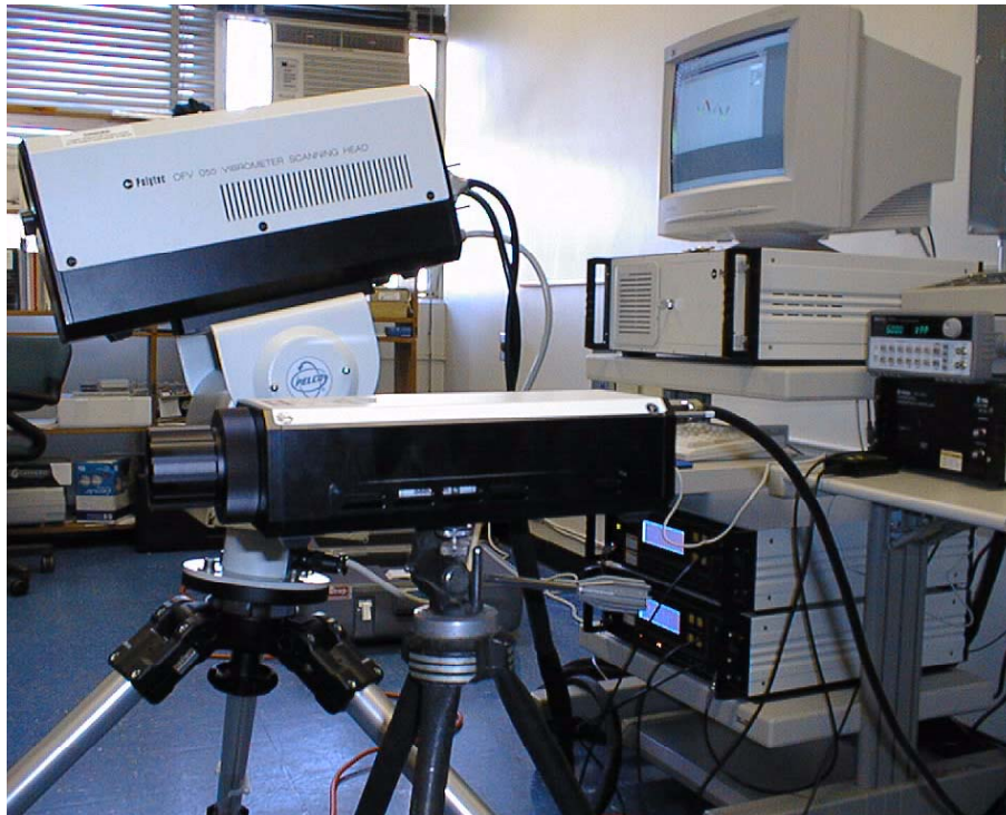
Figure 3-11. The SLDV system
