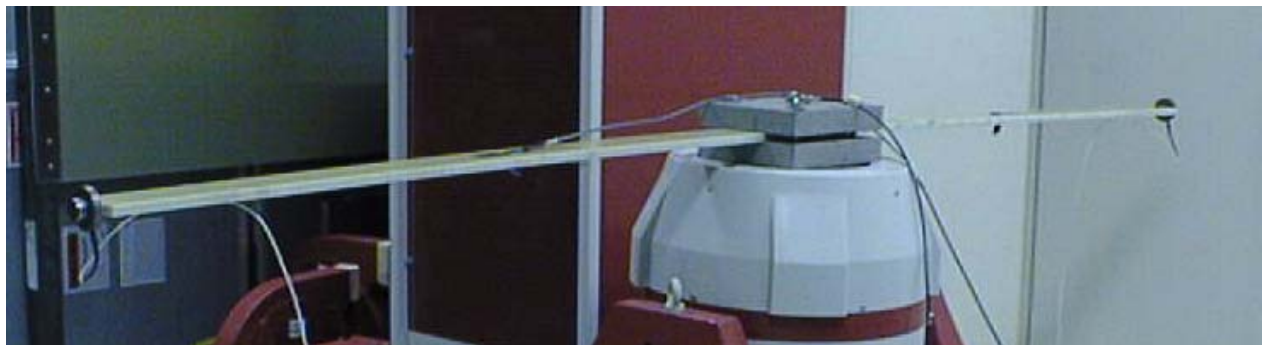
Figure 3-17. Composite beams used for damage detection testing
