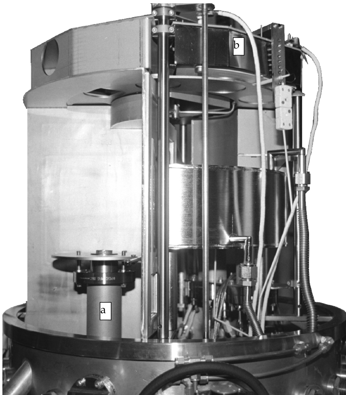
Figure 3-3 Detail of the chalcogen (selenium and/or sulfur) deposition zone of the reactor with the chamber outer walls removed, showing a) effusion source before the plasma cracker is mounted on the left and b) radiant heater with power leads and monitoring thermocouple at top right.
