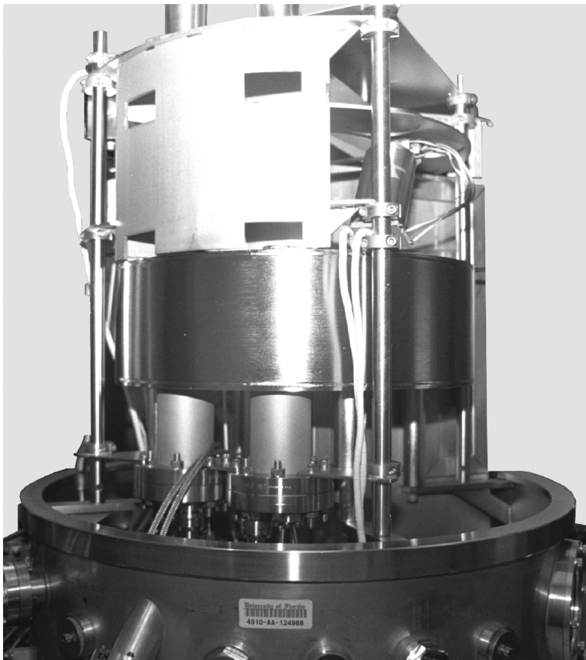
Figure 3-2 Detail of metals deposition shield with chamber removed.
