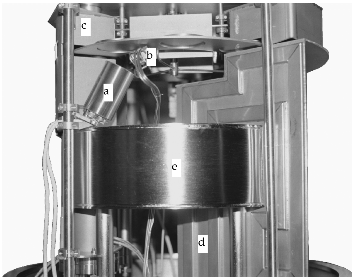
Figure 3-4 Detail of reactor viewed from the front load-lock zone with the chamber walls removed. The NaF Knudsen cell source (a) and QCM (b) are visible at upper left, in front of the metals deposition shield (c). The water-cooled selenium sector shield (d) is on the right and the annular liquid-nitrogen cryoshroud (e) at center.
