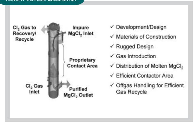
The success of the cell feed purity project, along with extensive testing of experimental equipment, helped in the design of a new electrolyzer that was compatible with the improved MgCl<sub>2</sub> feed. The new electrolyzer was also designed to provide:
