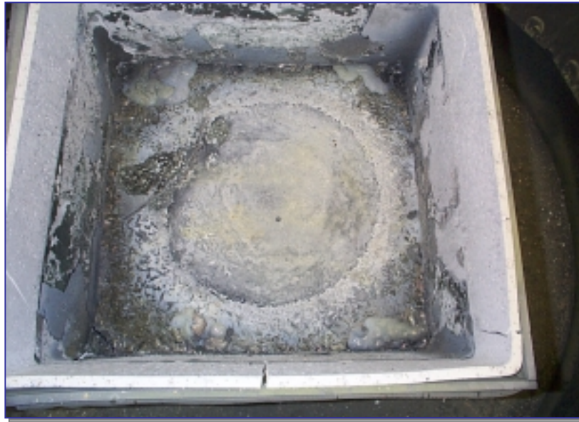
Figure 10. A 60-kg MG silicon charge after refining during Run MG3-10.
