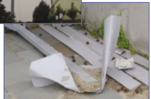
Figure 19. The Evans Residence turbine fell after a guy wire failed. Here you see the tail crushed with embedded rocks and soil. Next to it lay the blades.
