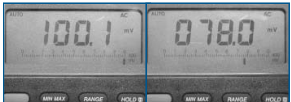
Figure 2: Current indicated by current transducer with fully closed jaws (left) and 40-millimeter gap (right) with constant load (1 millivolt/amp scaling).
