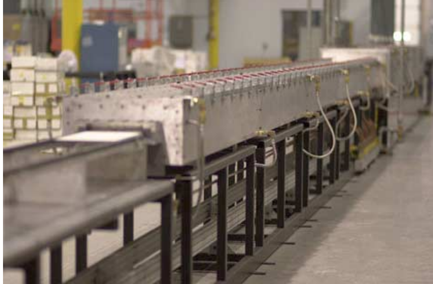
Figure 3. SF5 Silicon-Film™ sheet generation system. This single system has a capacity of 15 MW per year.
