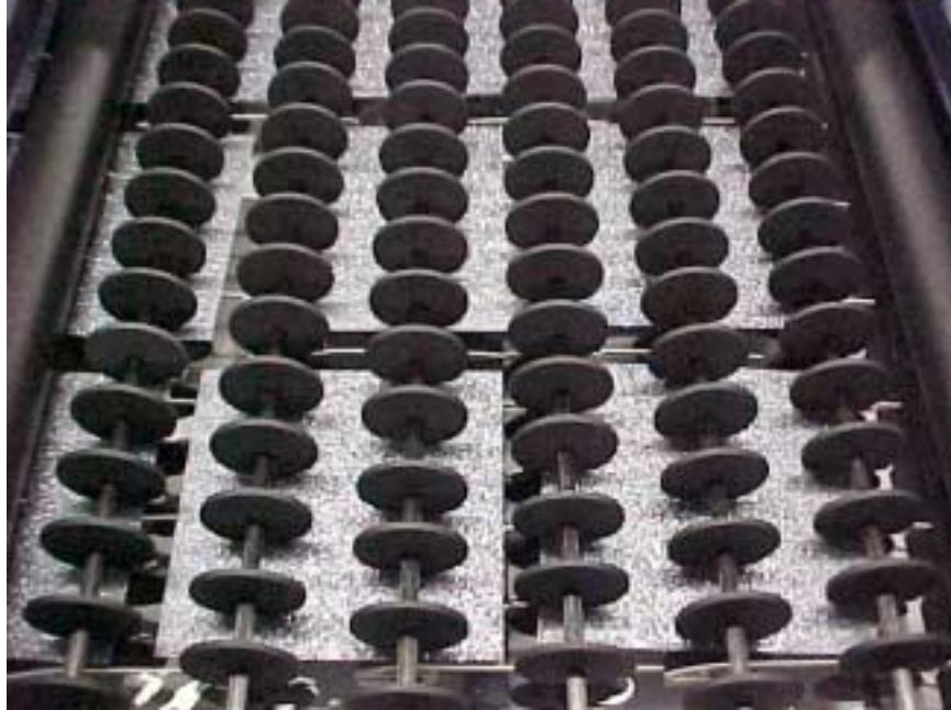
Figure 6. In-line diffusion oxide etch system. AP-225 Silicon-Film™ wafers in HF immersion etch module
