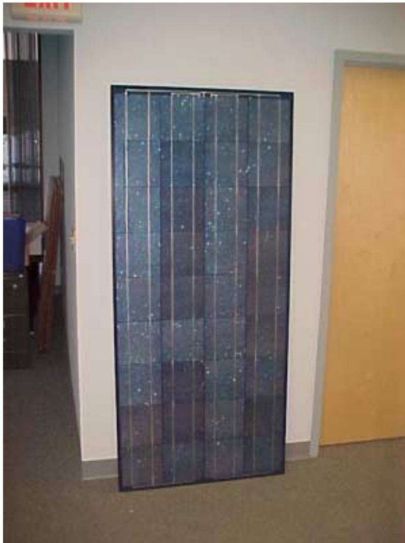
Figure 12. APx-150 module assembled with APx-8 Silicon-Film™ solar cells.
