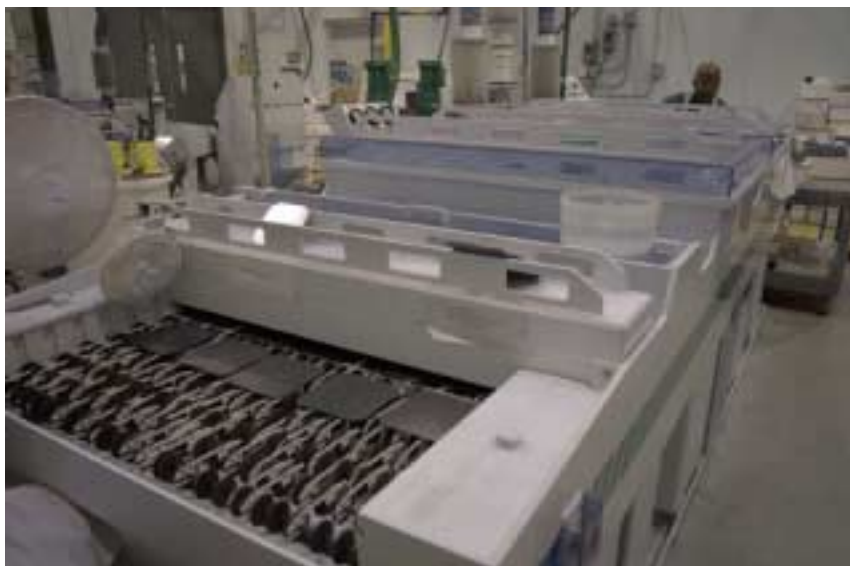
Figure 7. Continuous diffusion oxide etch system, unload end view.
