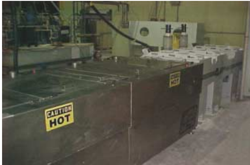
Figure 8. New continuous in-line sodium hydroxide etch prototype.
