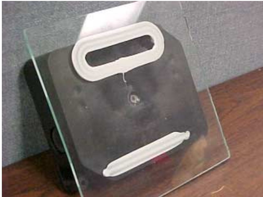
Figure 16. Junction box adhesive glueline example.
