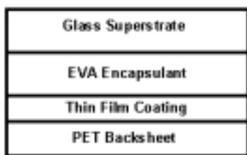
Fig. 1. A schematic of the test module construction used throughout the accelerated testing environments. PV devices are normally located between the glass and EVA.
