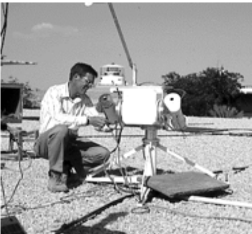
Figure 8.2. All-weather absolute cavity radiometer (right) and shaded infrared radiometer (top left) on BSRN Brusag tracker at the Solar Village.
