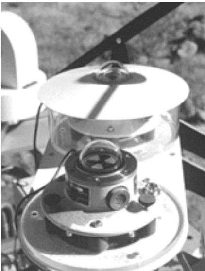
Figure 4.1. All-black (top unit) and black and white thermopile pyranometers under tracking shading disks.
