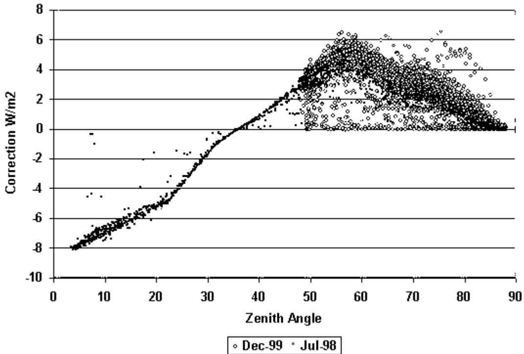
Figure 4.6. Absolute magnitude of corrections in global horizontal irradiance ( W/m^2 ) data measured with composite responsivity as a function of zenith angle for December (open circles) and July (points) at Qassim.
