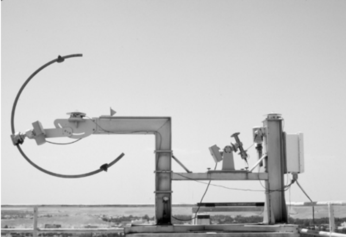
Figure 2.2. Profile of Saudi Arabian Instrumentation Platform. Instruments (left to right) are tracking shading disk, diffuse (shaded) pyranometer, north-south alignment sight, Normal Incidence Pyrheliometer in ST-1 Tracker, temperature and relative humidity sensor housing, global horizontal pyranometer, and data logger environmental housing.
