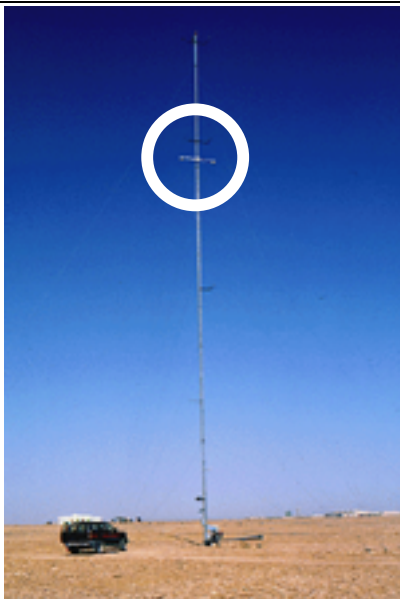
Figure 8.4. Tower installation for upwelling shortwave and longwave radiometers. Radiometers mounted on cross arms (inside circle) at 30 m above ground.
