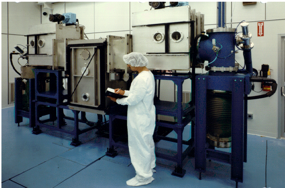
Fig. III-1. United Solar's roll-to-roll backreflector machine. This machine is also part of United Solar's decommissioned 2 MW plant and will be used for the bulk of Task 3, and for part of Task 7.
