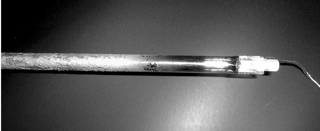
Fig. I.1. Photograph showing the IR lamps coated with deposition material.
