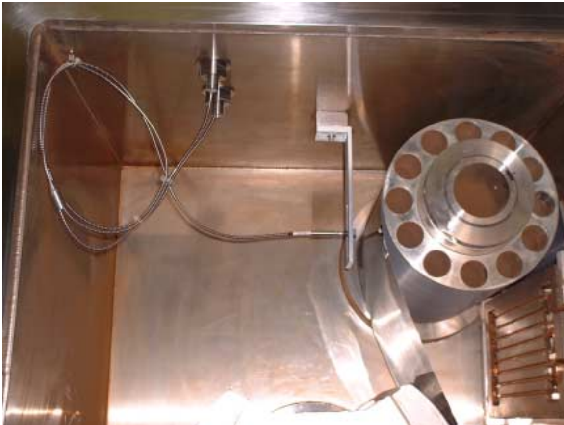
Fig. II.C-13. Spectrometer fibers mounted in a-Si Take-Up chamber.
