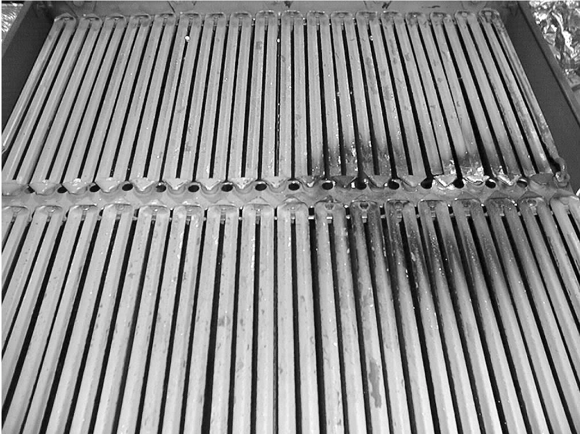
Fig. I.6. Photograph of failed heater assembly.
