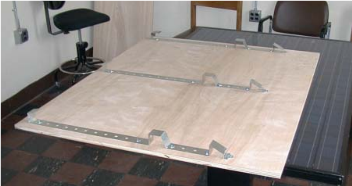
Figure 10: Sloped Tile Base Strips
