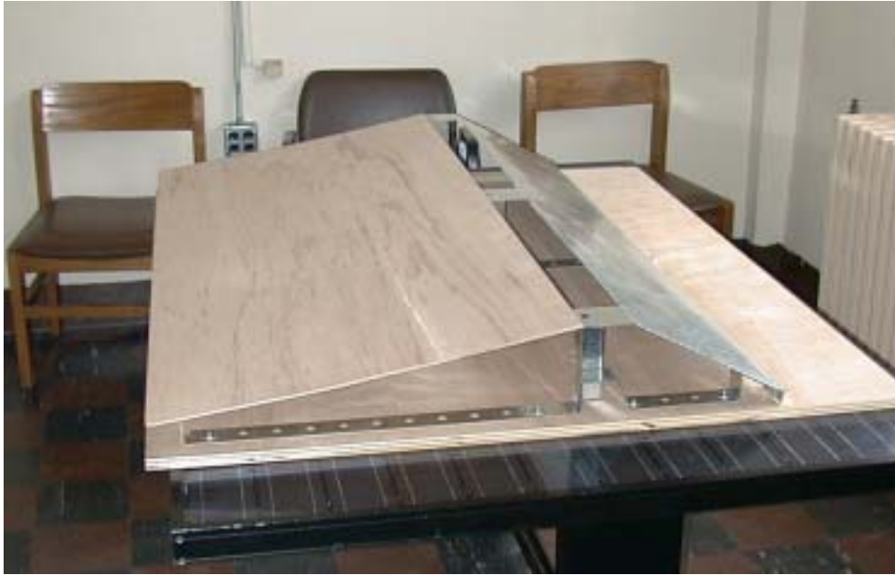
Figure 11: Sloped Tile Base Strips and Deflector Completely Assembled
