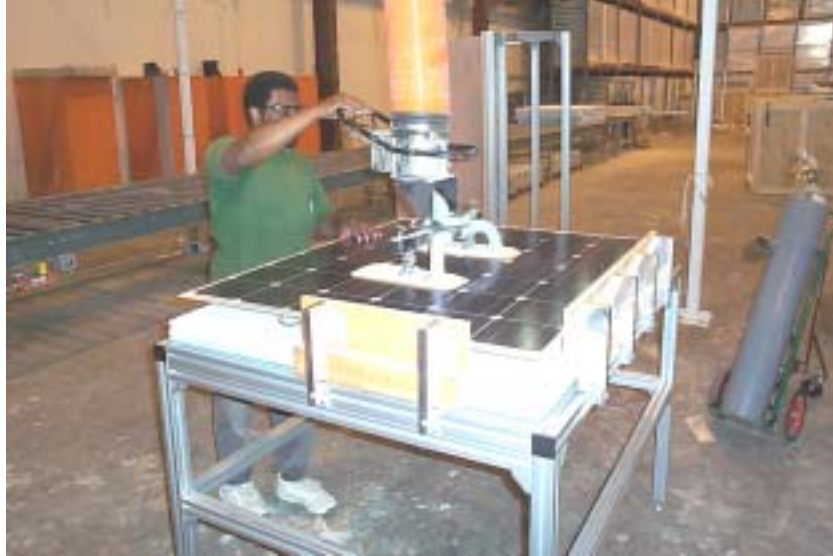
Figure 2: Laminate Placed on Backerboard
