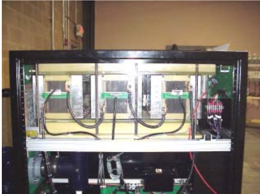
Figure 2-10. Left view of the fuel cell cabinet showing the three fuel cell stacks
