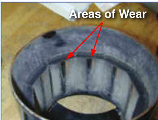
Figure 5. The inside of the magnet can.
